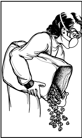
Figure 2: Wear protective clothing when installing insulation.
